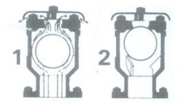
During the exhausting sequence, the air flowing around the buoy ball produces a resultant downward force which maintains the ball in the open position.
